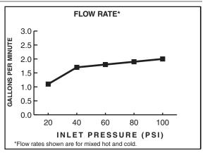
2.2 gpm/8.3 L/min. FLOW RATE
