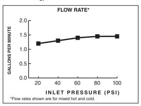
1.5 gpm/5.7 L/min. FLOW RATE
